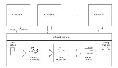
Figure 3: Architecture of the network simulation layer.
