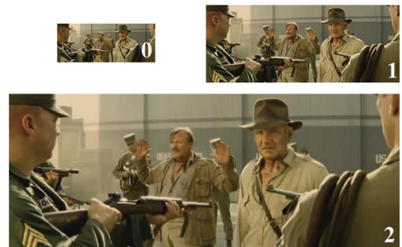
Fig. 1. Spatial scalability with three spatial layers. The resolution doubles with each layer.
