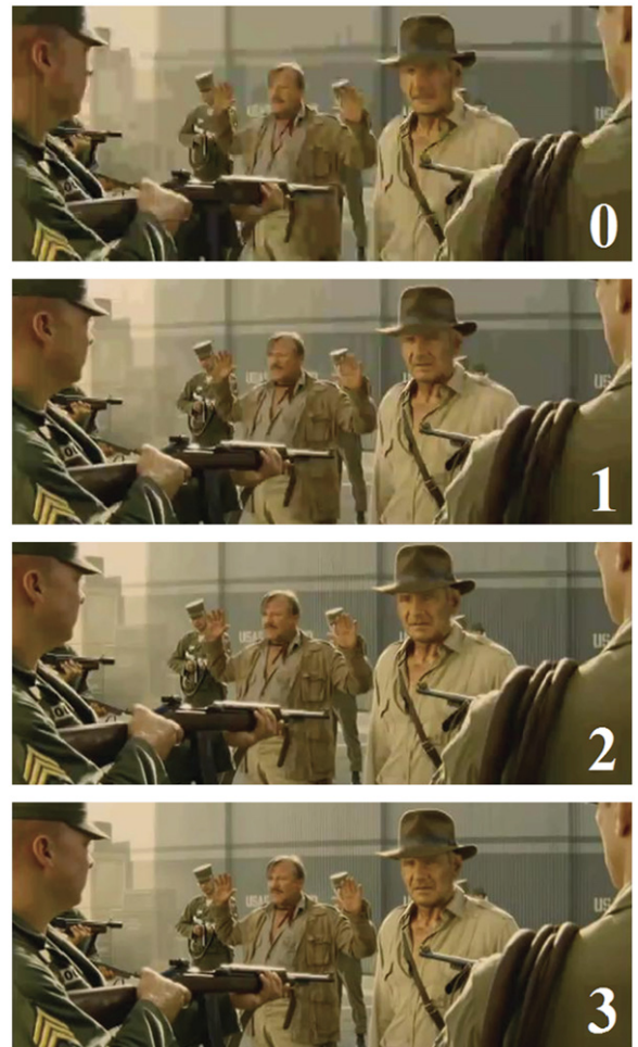
Fig. 3. Quality scalability with four quality layers. The picture quality increases with each layer; the resolution remains the same. The H.264 quantization parameter QP is decreased by 6 with each layer.
