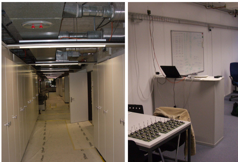
Figure 3.3: Left: During the benchmarking of the Dozer system our office building was under heavy construction work leading to additional interference. Right: To increase the communication range of the base station it was mounted on a cable rack about 2 meters above the floor.
