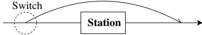
Fig. 2: Pods can switch tubes at stations without passing through an air lock.
