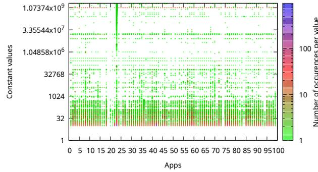
**Fig. 3.** Distribution of 32-bit constant values encountered during transformation. Apps are taken from the list of most popular applications on Google Play. Constants within the interval  $[-9, 9]$  are ignored.
