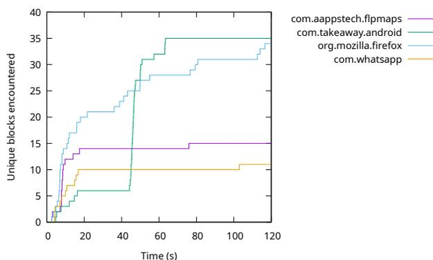
**Fig. 6.** Unique blocks encountered while running a few apps from Google Play while providing a random input every 100 ms for 2 minutes using Monkey.
