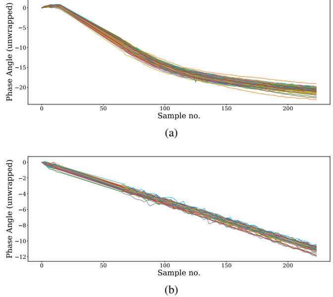
Fig. 2: Phase patterns of multiple messages from two different aircraft.
