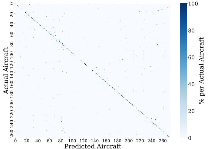
Fig. 4: Confusion matrix for aircraft classification when combining preamble phase and phase patterns
