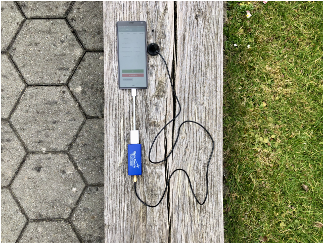
Figure 6: The evaluation setup consists of an Android smartphone with an RTL-SDR receiver attached to it.
