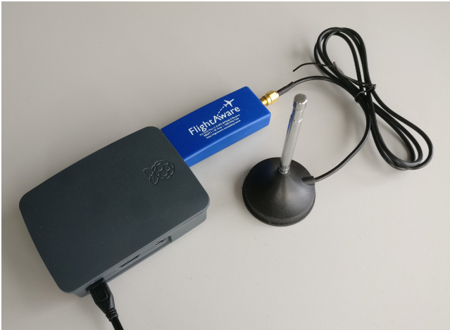
Figure 4: Hardware of ground station: Raspberry Pi 3 with FlightAware Pro Stick Plus and antenna. The Raspberry Pi decodes the messages and sends them to the server via LAN or WLAN.
