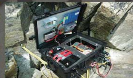
Base station power supply, system monitoring and a backup GSM modem are housed separately
