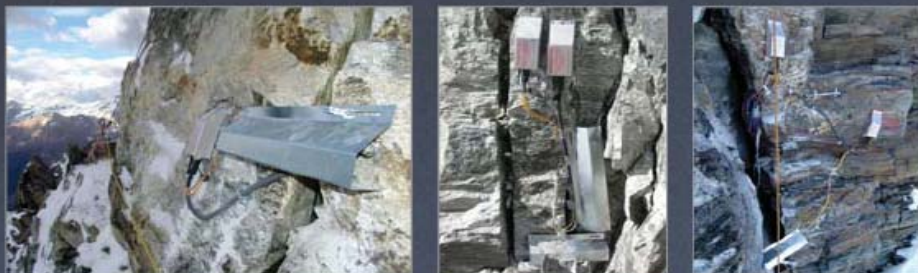
Sensor node installations targeting 3 years unattended lifetime
