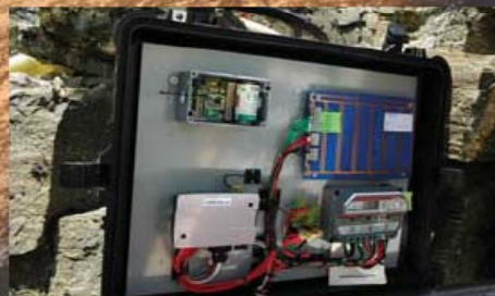
Base station power supply, system monitoring and a backup GSM modem are housed separately
