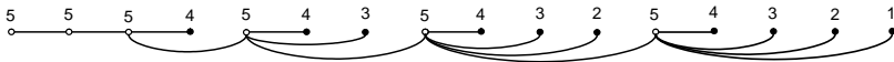
Figure 17.4: The interference of the exponential node chain—shown in a logarithmic scale—is bounded by O(\sqrt{n}) by the topology control algorithm \mathcal{A}_{exp} . Only hubs (hollow points) interfere with the leftmost node. For clarity of representation, some edges are depicted as curved arcs.
