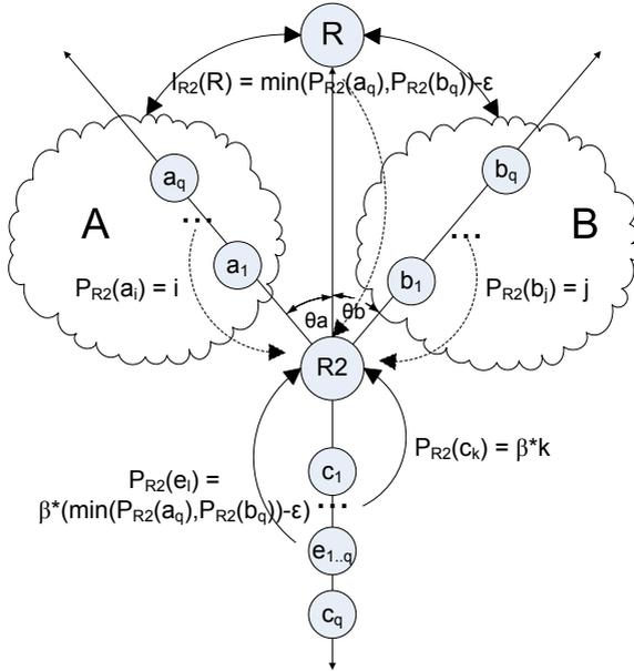
Figure 8.2: Reduction from NMTS: all  $4q$  links can be scheduled successfully in  $2q$  time-slots if and only if senders  $a_1, \dots, a_q, b_1, \dots, b_q, c_1, \dots, c_q$ , are partitioned into  $q$  triples  $(a_i, b_j, c_k)$  such that  $(i + j) = k$ .
