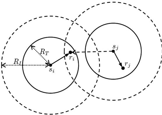
Figure 2.2: Protocol interference model: there are two radii: transmission range  $R_T$  and interference range  $R_I$ . In this example, node  $r_i$  is not able to receive a transmission from node  $s_i$  if node  $s_j$  concurrently transmits to node  $r_j$ —even though  $r_i$  is not adjacent to  $s_j$ .
