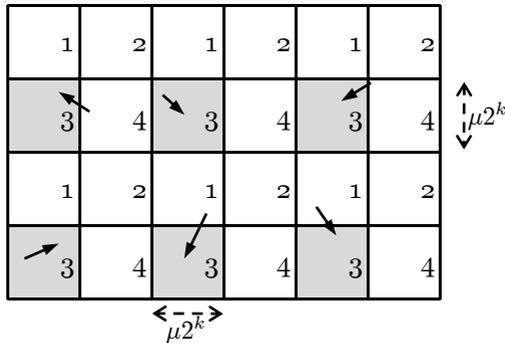
Figure 5.1: In line 11 of Algorithm 1, the algorithm picks all squares colored with color  $j$ . The example shows an inner loop iteration for length class  $G_k$  and  $j = 3$ . The algorithm schedules one unscheduled link from each selected square (if there exists one).
