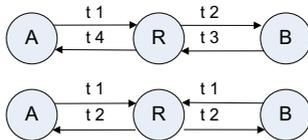
Figure 8.1: Analog network coding by signal mixing.
