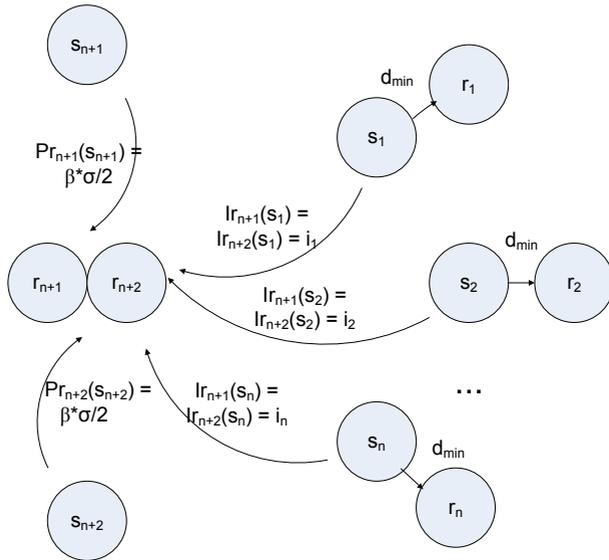
Figure 4.1: Reduction from Partition: link  $l_{n+1}$  (or  $l_{n+2}$ ) can be scheduled if and only if the interference caused by simultaneously scheduled links  $s_j, j \in \{1 \dots n\}$  is less or equal to  $\sigma/2$ .
