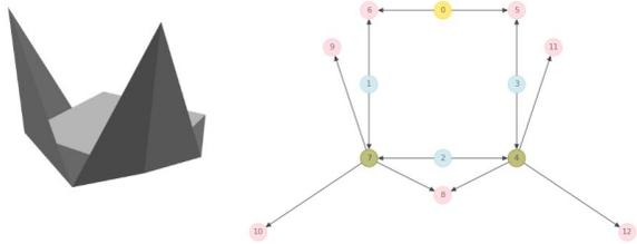
Figure 6: Seeding pattern for the chair fold. Left: the folded shape of the seeding pattern on its own. Right: The graph of the seeding pattern.
