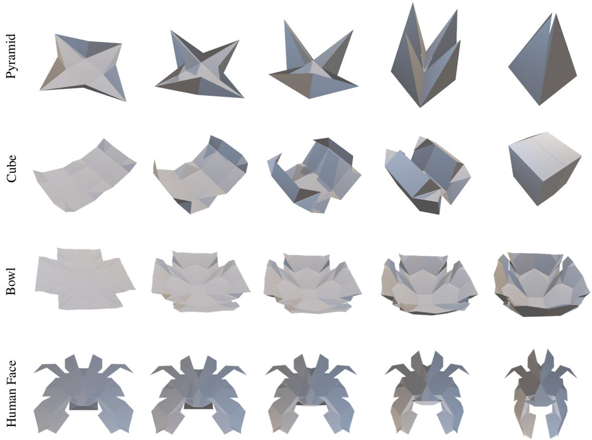
Figure 9: The folding motion of the best approximations for the four targets.
