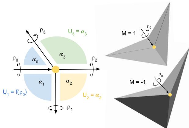
Figure 1: A degree 4 vertex with one incoming and 3 outgoing edges. Indicated are the sector angles  $\alpha$ , the folding (dihedral) angles  $\rho$  and the unit angles  $U_1$ ,  $U_2$  and  $U_3$ . The illustrations on the right show the effect of the rigid body mode  $M \in \{-1, 1\}$  for the same input angle  $\rho_0$ .
