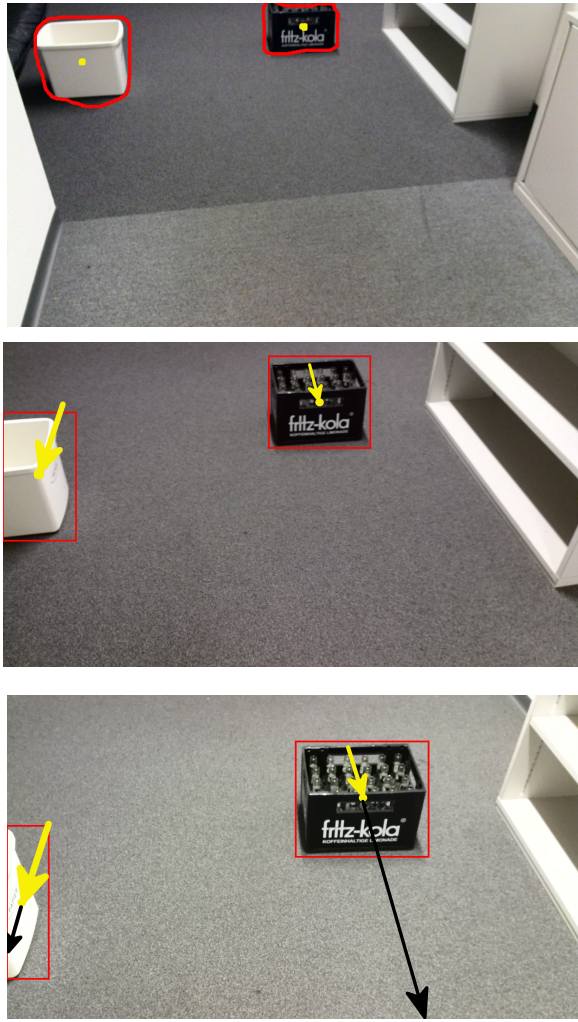
Figure 3: The yellow arrows depict the movement of the centers of masses of the objects and the black arrows correspond to the point where the object will go out of the field of view. The tracked objects are denoted by a red rectangle and their centers of mass are shown with a yellow circle. Since the movement of the trash bin is going left of the picture, we consider this object as harmless. The general direction of the fritz-kola case is towards the user and therefore a warning is thrown.
