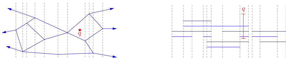
Fig. 1. (a) Planar point location problem. (b) Stabbing range query q on a set of n horizontal line-segments.
