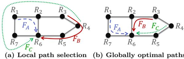
**Figure 2: Inefficient routing due to local allocation.**
