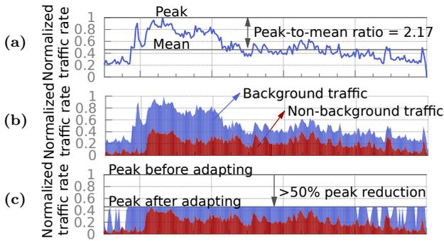
**Figure 1: Illustration of poor utilization.** (a) Daily traffic pattern on a busy link in a production inter-DC WAN. (b) Breakdown based on traffic type. (c) Reduction in peak usage if background traffic is dynamically adapted.
