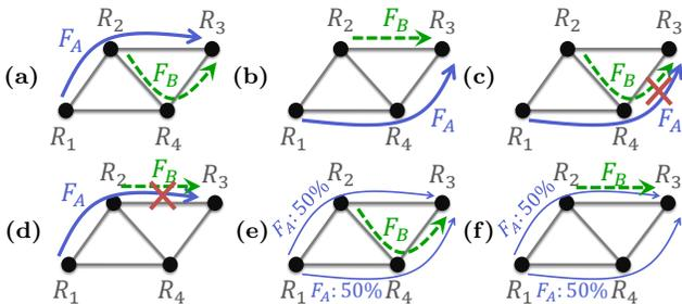
**Figure 4: Illustration of congestion-free updates.** Each flow’s size is 1 unit and each link’s capacity is 1.5 units. Changing from state (a) to (b) may lead to congested states (c) or (d). A congestion-free update sequence is (a)→(e)→(f)→(b).
