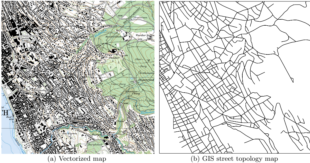
Figure 3: Vectorized map of downtown Zurich (left) and the associated GIS street topology (right). Maps are reproduced with authorization by Swisstopo (BA071556).
