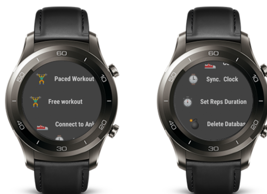
Figure 2. Main menu screen. Participants choose the workout type and set the vibration interval duration.
