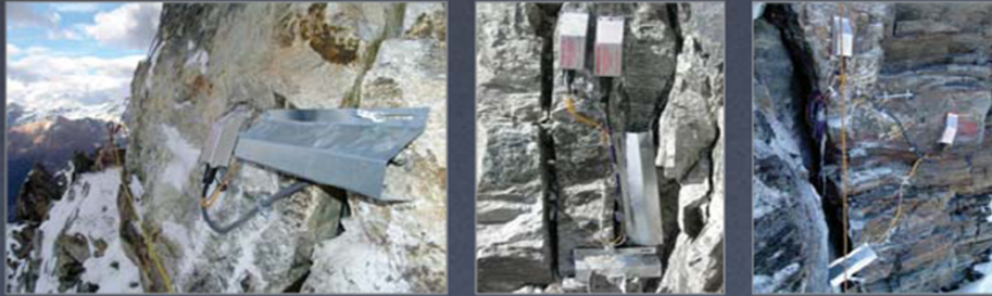
Sensor node installations targeting 3 years unattended lifetime
