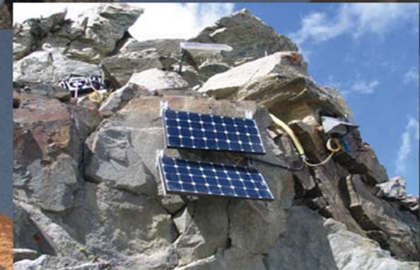
Base station and solar panels on the field site at Matterhorn
