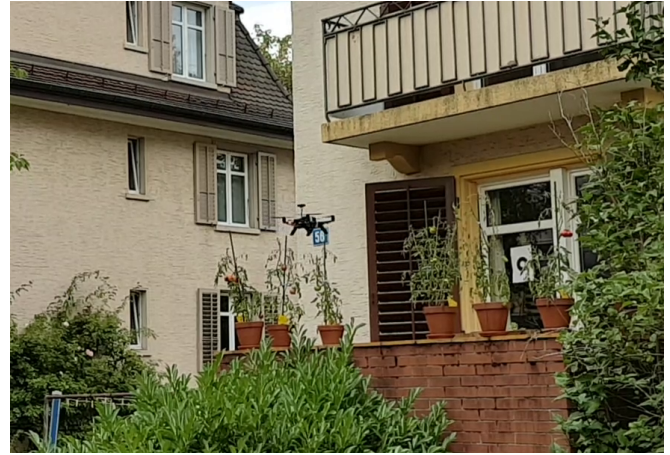
Fig. 8. Snapshot of the drone approaching the visual marker on a balcony during a field test.
