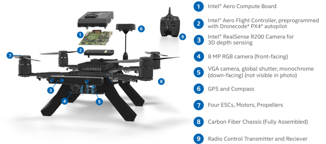
Fig. 2. Hardware components of the Intel ® Aero Ready to Fly Drone [16]. This drone is a fully-assembled, flight tested, ready to fly quadcopter intended to alleviate some of the development burden from commercial drone developers and researchers.
