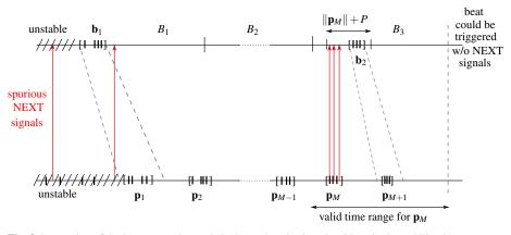
**Fig. 3** Interaction of the beat generation and clock synchronization algorithms in the stabilization process, controlled by Algorithm 4. Beat  $\mathbf{b}_1$  forces pulse  $\mathbf{p}_1$  to be roughly synchronized. The approximate agreement steps then result in tightly synchronized pulses. By the time the nodes trigger beat  $\mathbf{b}_2$  by providing NEXT signals based on  $\mathbf{p}_M$ , synchronization is tight enough to guarantee that the beat results in no resets.
