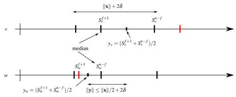
Fig. 1 An execution of Algorithm 1 at nodes v and w of a system consisting of n=4 nodes. There is a single faulty node and its values are indicated in red. Note that the ranges spanned by the values received from non-faulty nodes are *almost* identical; the difference originates in the perturbations of up to  $\delta$ .
