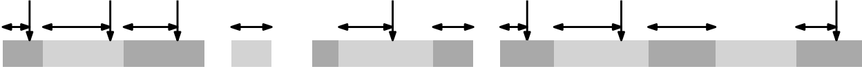
Figure 1: A realization of an alternating Poisson process with time progressing from left to right. The dark gray, light gray, and white intervals represent the colors 1, 2, and \perp , respectively. The vertical arrows represent the meaningful alternation times and the horizontal two-sided arrows depict the time intervals that contribute to the digestion of the corresponding iterations.
