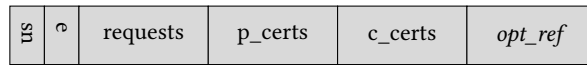
Fig. 9. Data structure format of PACK (known as block). A PACK consists of a sequence number sn , an epoch number e , a list of requests requests (to allow for batch-processing of requests), prepared certificates p\_certs of replicas having prepared this PACK, commit certificates c\_certs of replicas having sent a COMMIT message and an optional back-reference opt\_ref , if a PACK refers to another PACK (this is mainly used for hanging requests during epoch-changes).
