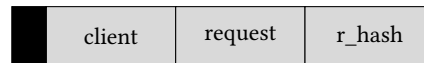
Fig. 16. Message format of REQUEST. It consists of the client’s unique identifier client , the request request and the hash of the request r\_hash .
