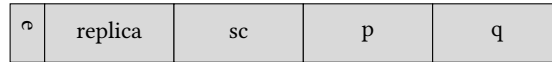
Fig. 10. Data structure format of EPOCHCHANGEOBJ. An epoch-change object consists of an epoch number e , an unique identifier replica and maps sc , p and q .
