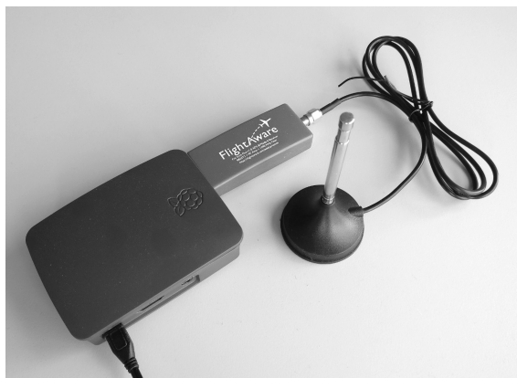
Figure 8.4: Hardware of ground station: Raspberry Pi 3 with FlightAware Pro Stick Plus and antenna. The Raspberry Pi decodes the messages and sends them to the server via LAN or WLAN.
