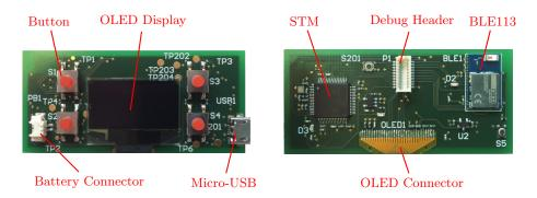
Fig. 4. The top and bottom views of the PCB.
