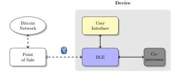
Fig. 2. System overview with contributing components.
